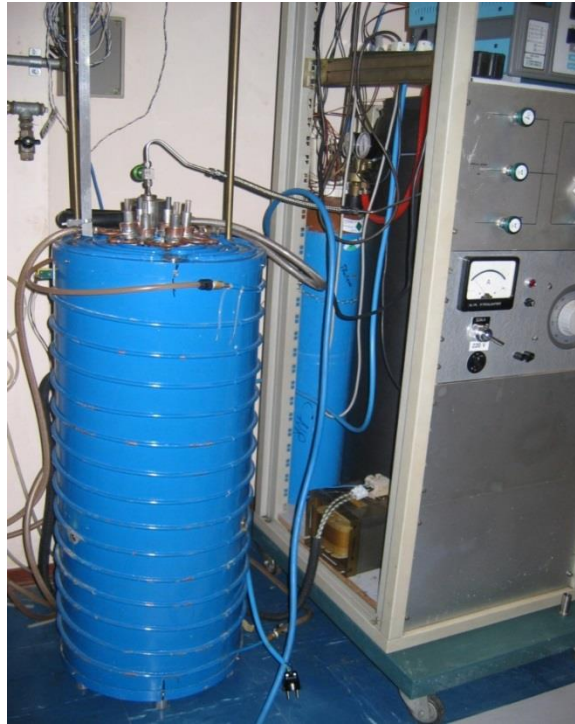
Figure 7. GCHP filled with potassium for calibration at INRiM. The system is equipped with a commercial pressure controller [3].
