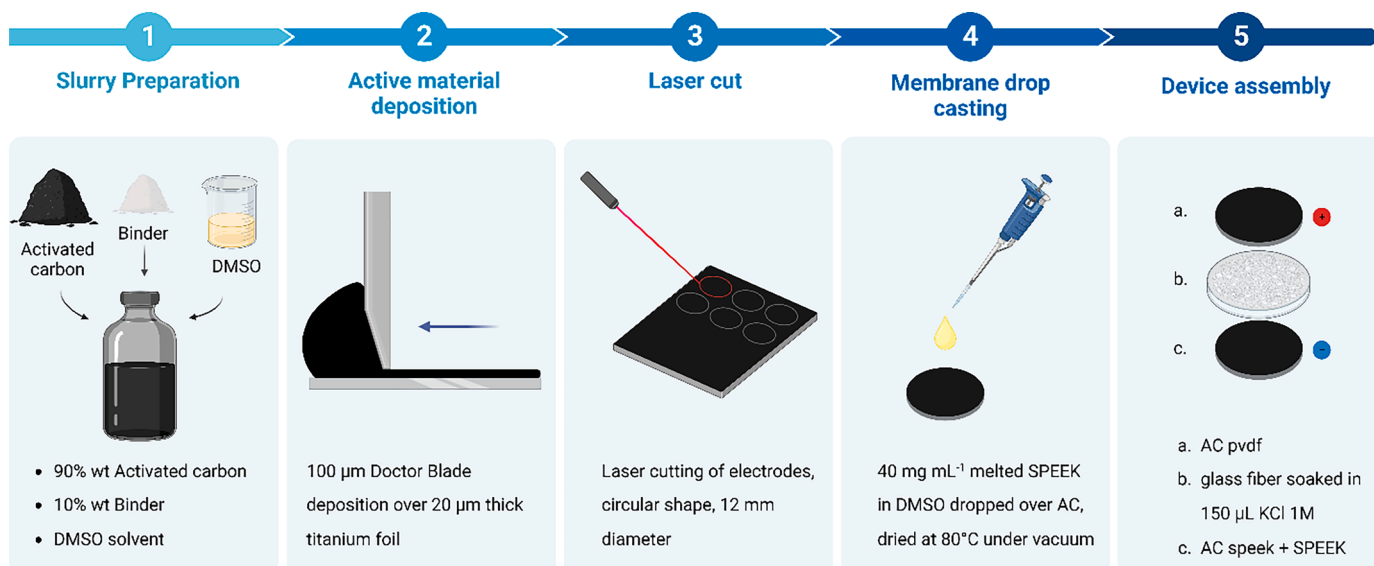
Fig. 2. Flowchart of electrodes and device production process.
