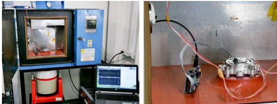
Figure 12: Experimental set-up for calibration by comparison in temperature controlled conditions.
