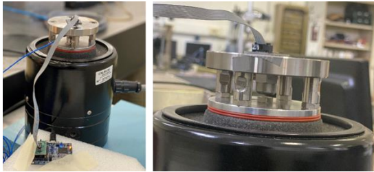
Figure 2: Calibration set-up by comparison with a reference accelerometer (PCB model 080A199/482A23), mounted below a supporting table, at INRIM.
