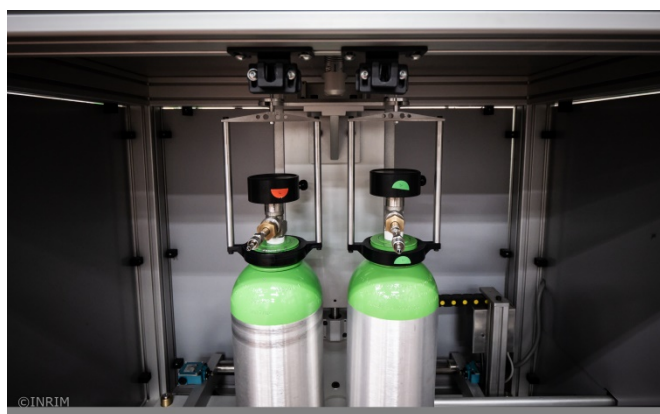
Fig. 2: Detail of the INRIM weighing device that allows the automatic exchange of the target cylinder and the tare without any intervention of the operator after the weighing process has started.
