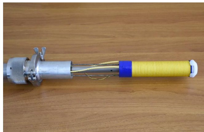
Figure 2. The probe cryomagnet, showing the yellow winding insulation. A header (white) was added to ease the insertion in the cryostat.
