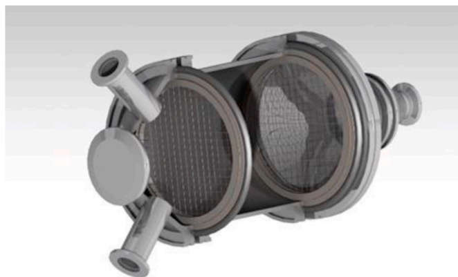
Fig. 1. Design of the mixing chamber of the dilution system (counter-flow inlets not shown).
