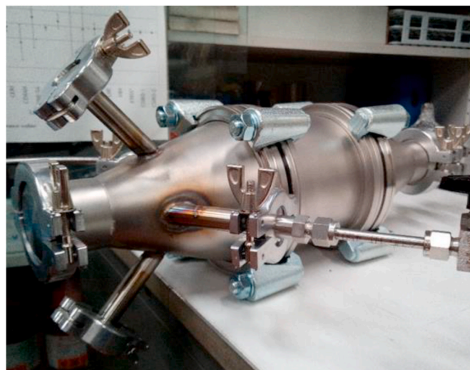
Fig. 2. The mixing chamber of the dilution system.
