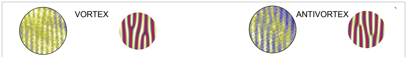
FIG. 4. Experimental and simulated interference pattern resulting after a Bragg interferometer applied on a BEC containing a vortex (left) or an antivortex (right).
