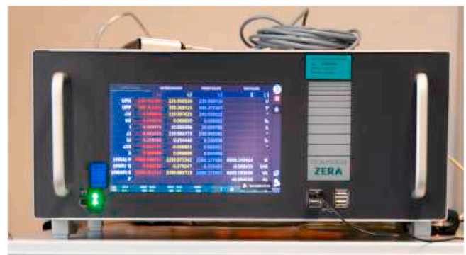
Fig. 3. The three-phase reference wattmeter/energy meter W_{REF} , a ZERA mod. COM5003.
