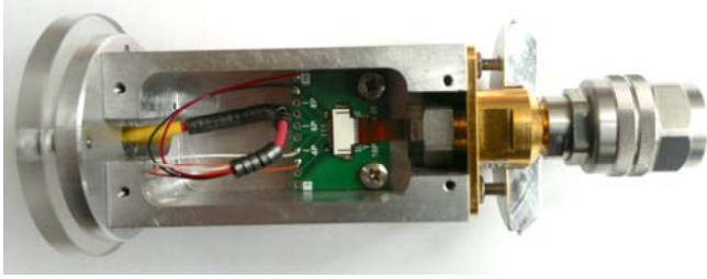
Fig. 1. Picture of the specific sensor mount under test.
