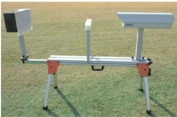
FIGURE 7 Image of the high-speed optical disdrometer Source: Testik and Rahman (2016)
