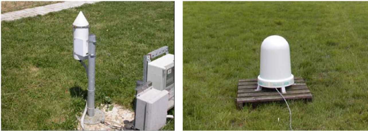
FIGURE 11 Microwave precipitation gauges: LCR PVK ATTEX on the left (from Cauteruccio et al., 2021a) and Pludix on the right (from Caracciolo et al., 2006)
