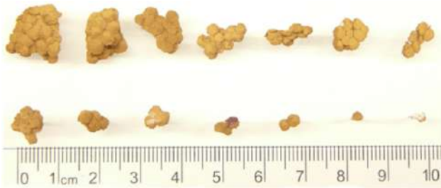
FIGURE 16 Image of the Styrofoam particles used by Bernauer et al. (2015) to simulate solid precipitation
