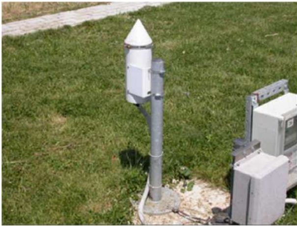
FIGURE 11 Microwave precipitation gauges: LCR PVK ATTEX on the left (from Cauteruccio et al., 2021a) and Pludix on the right (from Caracciolo et al., 2006)
