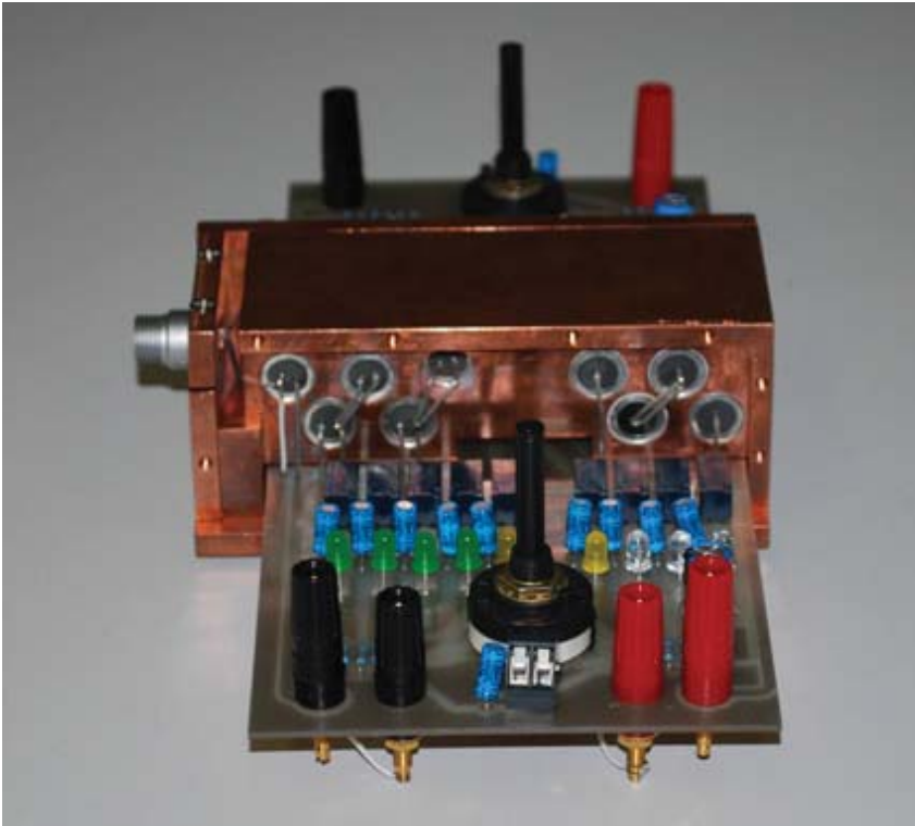
Figure 2. Photo of the INRIM divider in which the copper box housing the resistors can be seen.
