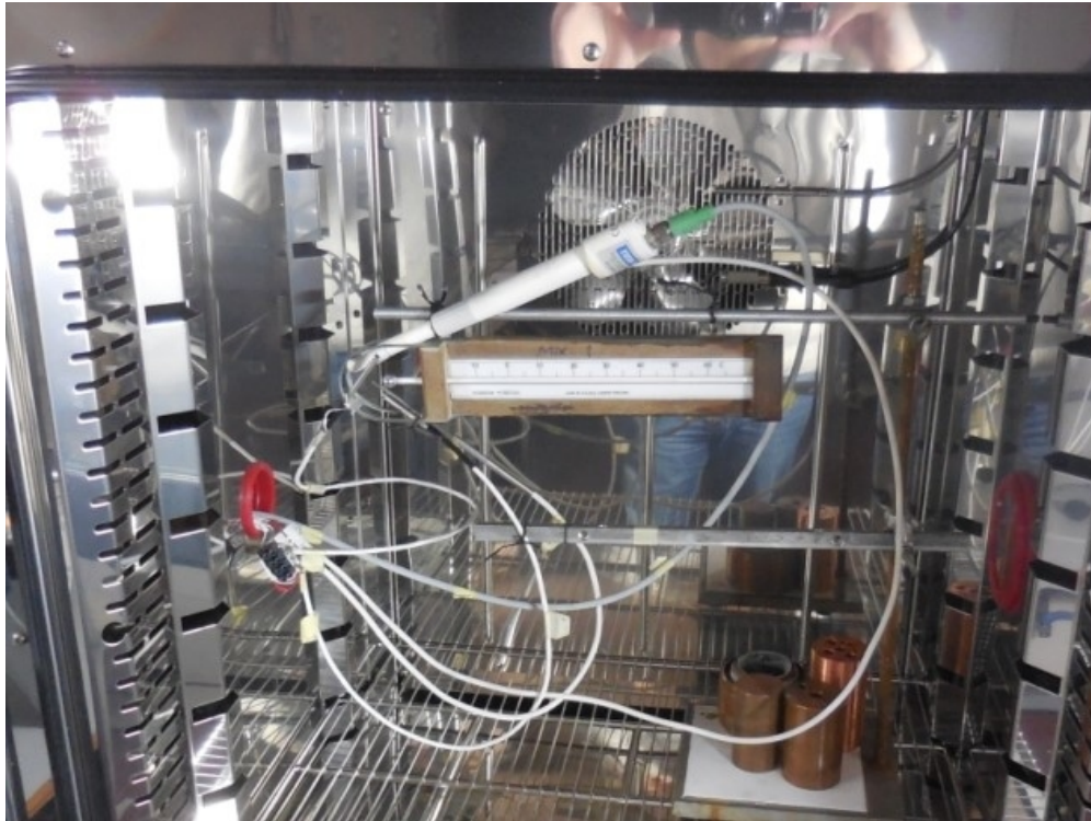
Figure 4. The Kuwait HMP155 and the Pakistan G.H.Zeal thermometers in the climatic chamber for comparison.
