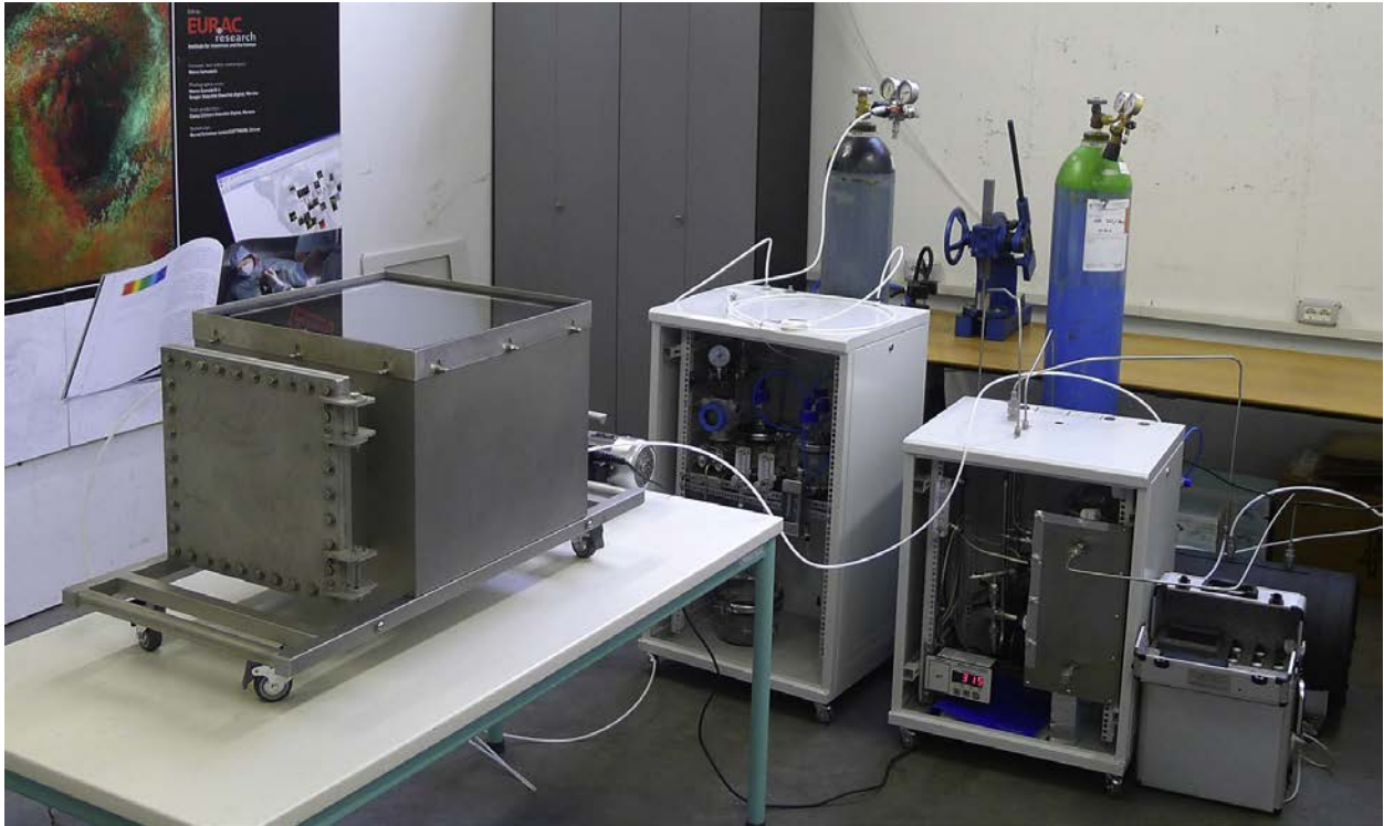
Fig. 2. Display case prototype connected to the O2 analyzer during the leak rate tests.
