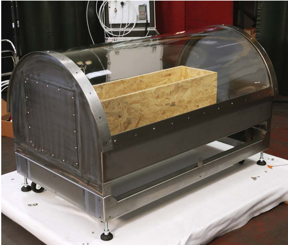
Fig. 1. Display case prototype for the mummy of Rosalia Lombardo (1918–1920AD), Palermo, Italy
