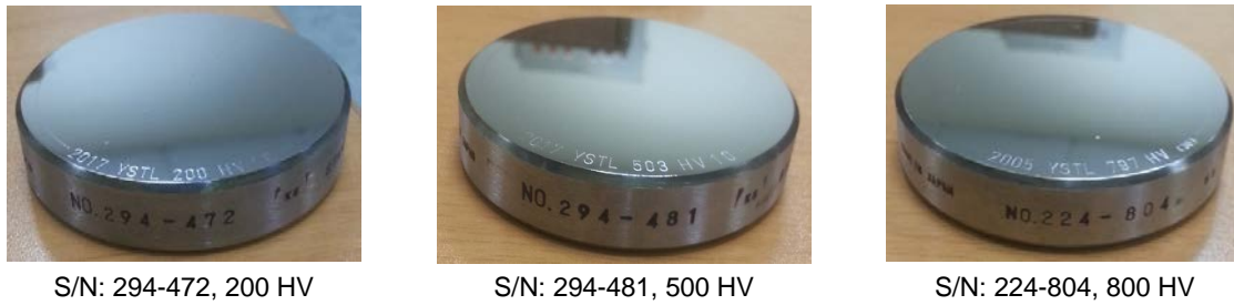
Figure 3. Transfer Standards for HV1 and HV30 Scales.
