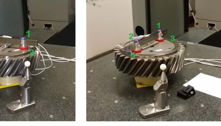
2. The second step performed the full measurement of the master, as well as a repetition of the measurement of the three pre-calibrated features. The *x* coordinates of all measured points were stretched (i.e. multiplied by a common factors close to unity) to make the repeated measurement value of the pre-calibrated *x* feature match the pre-calibrated value. The same was done separately for *y* and *z*.
