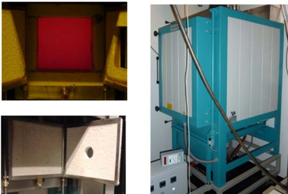
Figure 2 Facility for industrial size-of-source characterization developed at VSL.
