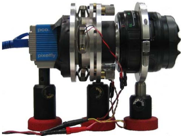
Fig. 1. The optical set-up formed by a photographic objective, on the right hand side, that forms the image of the scene on the CCD camera on the left hand side. In the middle the F-P interferometer. The three piezo actuators that change the optical path distance by moving the mirrors are visible in the aluminum structure.
