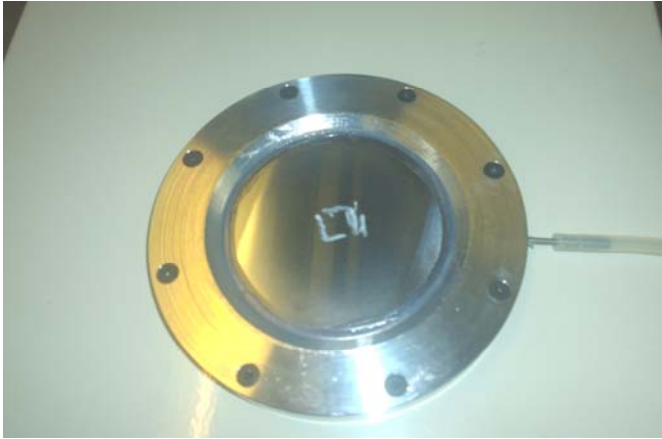
Fig. 4. The Fabry-Perot interferometer formed by two silicon wafers inserted in a sealed structure where the distance is varied with a pneumatic technique.
