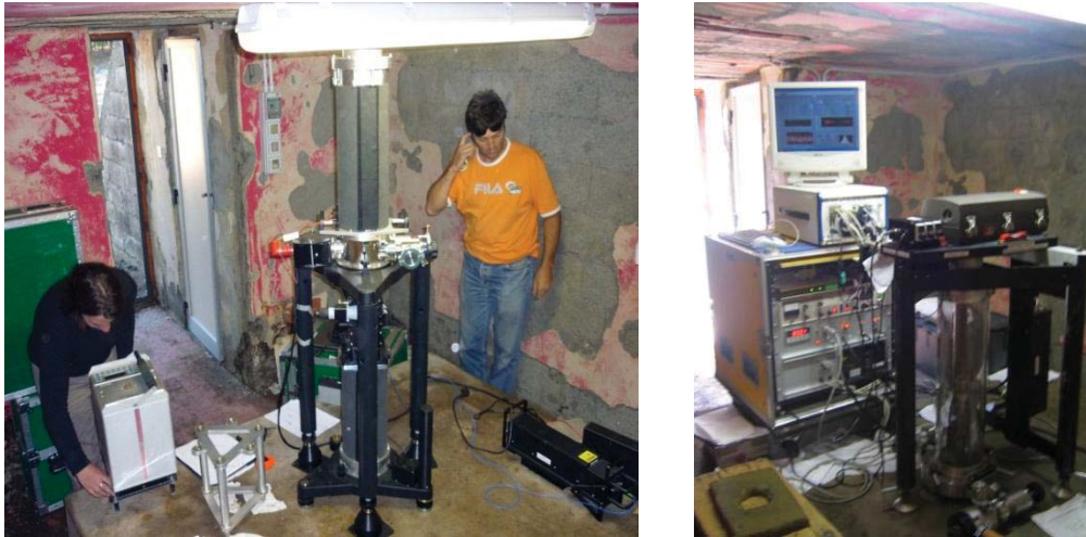
Fig. 2 – Gravity station at Serra La Nave (SLN, Mt. Etna): on the left the FG5#238, on the right the IMGC-02 during the measurements.
