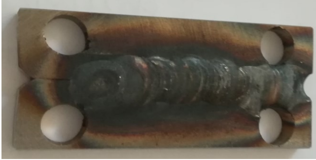
Fig.4. AISI sample welded by TIG
