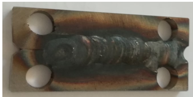
Fig.4. AISI sample welded by TIG
