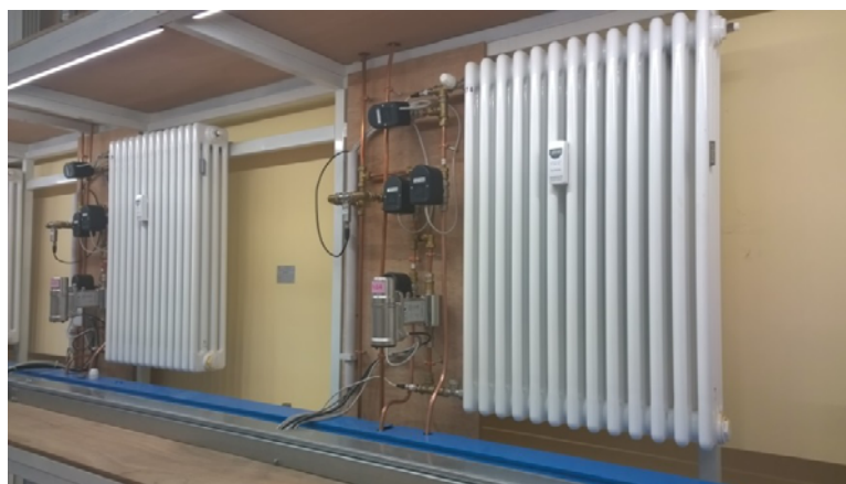
Fig. 12. HCAs installed at the INRIM thermo-hydraulic simulator.
