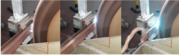
Fig. 5. Arc evolution on the wheel: (left) ignition, (middle) elongation, (right) quenching
