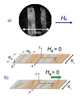
Fig. 7. Observed domain structure in the  $K_{\perp}$  nanocrystalline ribbon (a) and its schematic representation (b). The magnetic moments inside the transverse domains oscillate around the *x*-direction upon application of a longitudinal (y-axis) AC field  $H_a$ .
