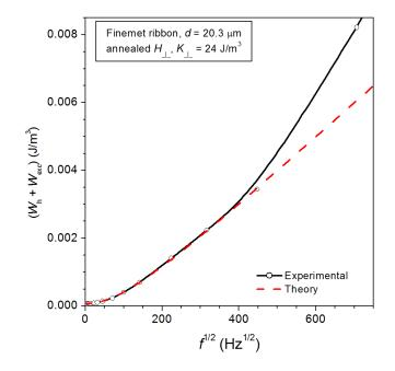
Fig. 6. The experimental quantity  $W_{\rm h} + W_{\rm exc}(f)$  in the transverse anisotropy Finemet ribbon is predicted by Eq. (3) up to  $f \sim 200$  kHz.
