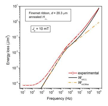
Fig. 8. Example of energy loss measured up to 1 GHz at  $J_p = 10$  mT in the  $K_{\perp}$  nanocrystalline ribbon and theoretical prediction of the rotational contribution using: 1) The classical model  $(W_{\text{rot,Mxw}}(f))$  based on the Maxwell's diffusion equation with magnetic constitutive equation defined by  $\mu_{\text{DC}}$  (Eq. (2), dashed line); 2) Modeling by coupled Landau-Lifshitz and Maxwell's diffusion equation  $(W_{\text{rot,LL}}(f), \text{Eq. (19) solid line)}$ .
