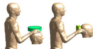
Fig. 6. Model of the operator body with respect to the patient head. One positions (#3) has been considered for both coils, with and without shield.
