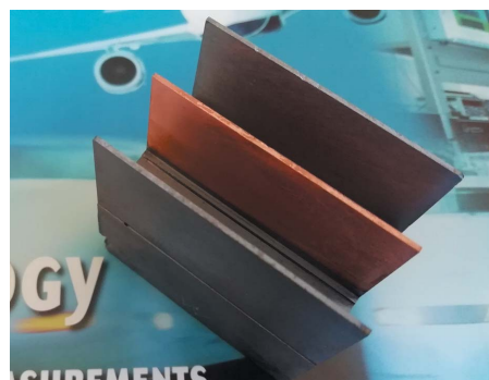
Figure 2 Photograph of the X-ray interferometer with a Cu film on the mirror crystal. The film thickness has been increased to make it visible.
