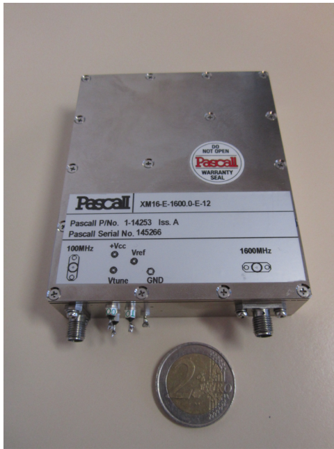
FIG. 2. Photograph of a 100 MHz-1.6 GHz XM16 Pascall frequency-multiplication module.
