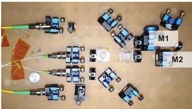
Fig. 3. Picture of the optical board and the mirrors for the stability and noise test. The two white fibers are the input radiations from the laser source; the two yellow fibers are the output radiation towards the detectors.
