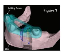
**Figure. 1**: Trial of a dental drilling guide produced by additive manufacturing for the drilling of holes to fit dental implants into artificial jaw models with only few abutment teeth. The drilling angle  $\alpha$  and the drilling depth were measured by means of computed tomography. Source: PTB
