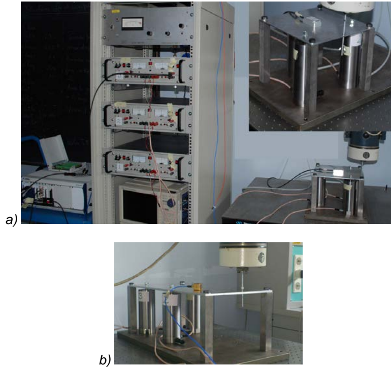
Figure 13. a) Details of the complete set-up. On the left, power electronics, acquisition, conditioning and control. On the right, a test-rig with the shaker. At the top right, details of the test-rig. b) Rectangular plate.
