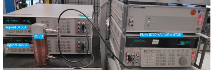
Fig. 8. Second method measurement setup for SF characterization of the RCVD up to 100 kHz.
