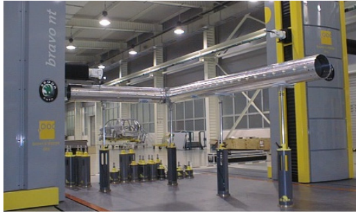
Figure 28. L-shaped dismantable artefact for large-scale metrology developed within the MESTRAL project [268].
