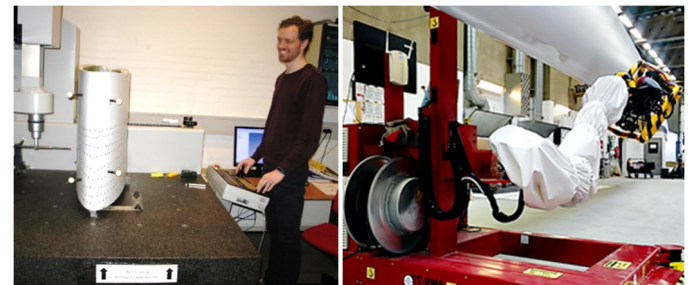
Figure 24. Establishment of the traceability of automated freeform optical scanner measurements on wind turbine blades in the production [199]. Left: calibration of freeform surface of a wind turbine blade section. Right: optical 3D scanner mounted on a 6 DOF robot with reference to a laser tracker during measurement of a 55 m wind turbine blade.
