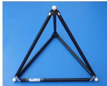
Figure 44. Ball tetrahedron artefact (source: Trapet Precision Engineering).
