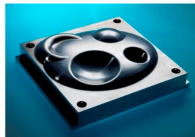
Figure 20. NPL freeform artefact [208]; the nominal dimensions of the model shown are 150 mm × 150 mm × 40 mm.
