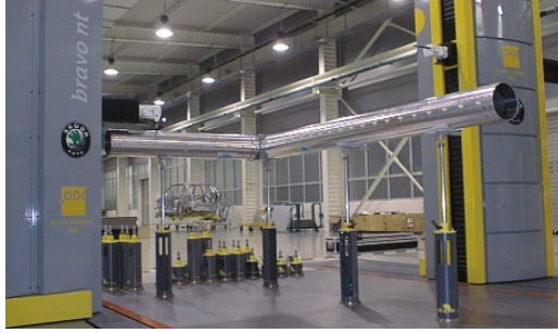
Figure 28. L-shaped dismountable artefact for large-scale metrology developed within the MESTRAL project [268].
