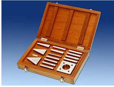
Figure 35. Set of angle gauge blocks (source: PTB).
