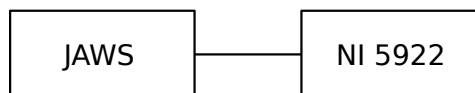
Figure 2.46: NI 5922 – Linearity – Advanced calibration connection where Josephson arbitrary waveform synthesizer (JAWS) is used as a reference.
