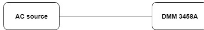
Figure 2.15: DMM 3458A - Frequency response - A simplified calibration connection where AC voltage source is used as a reference.
