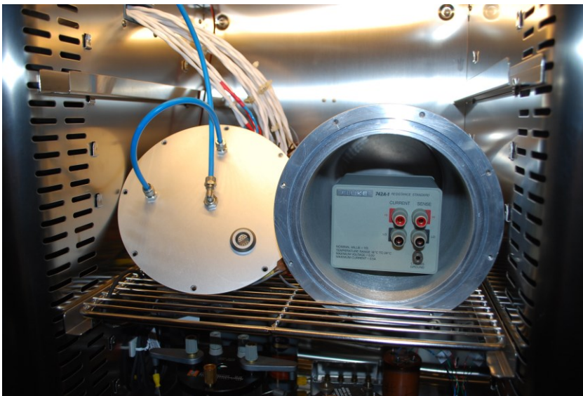
Fig. 3 - Case for the characterization of pressure and humidity in the air-bath whose stability is 0.01\text{ }^{\circ}\text{C} at T = 23.0\text{ }^{\circ}\text{C} . The humidity and pressure control systems are external.
