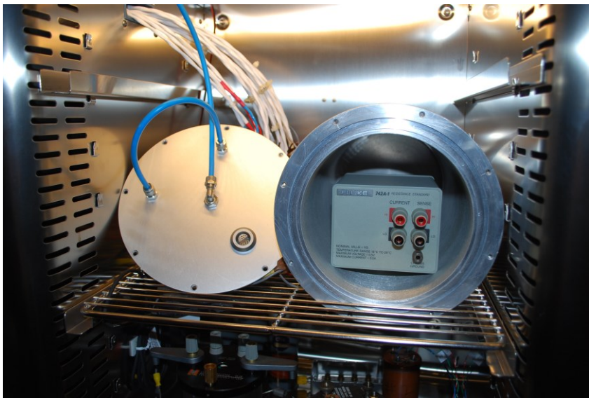
Fig. 3 - Case for the characterization of pressure and humidity in the air-bath whose stability is 0.01 °C at T = 23.0 °C. The humidity and pressure control systems are external.
