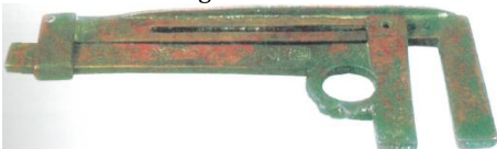
Fig. 3. Vernier caliper (9 AC) from Chinese Han dynasty [76].
