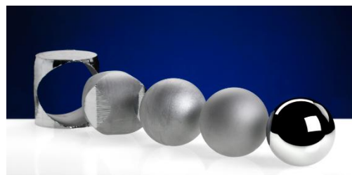
Fig. 29. Hollowed ingot, cut, turned, lapped and polished sphere [116].
