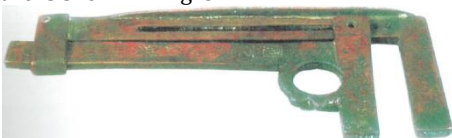
Fig. 3. Vernier caliper (9 AC) from Chinese Han dynasty [76].
