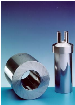
Fig. 46. Piston cylinder pressure gauge system [courtesy PTB].
