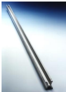
Fig. 8. Copy #23 of international metre prototype [courtesy PTB].
