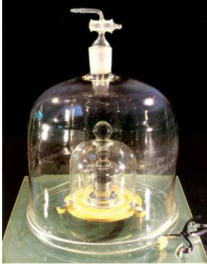
Fig. 10. International kilogram prototype [courtesy BIPM].
