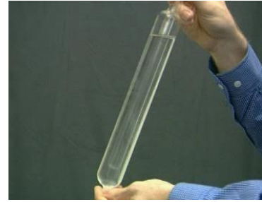
Fig. 12. A triple point cell of water [courtesy PTB].
