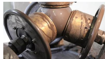
Fig. 28. Lapping tools of the tetrahedron lapping and polishing device designed and used in the PTB manufacturing chain for Avogadro spheres [courtesy PTB].
