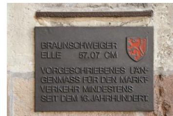
Fig. 5. 'Braunschweiger Elle', the local length standard mounted close to the Old Town Market of the city of Braunschweig, Germany [courtesy PTB].
