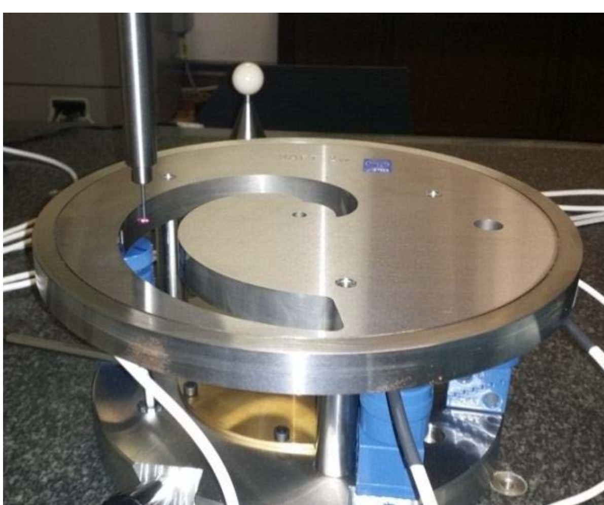
Example of internal involute measurement scanning
