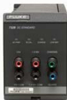
Fig.1. J. Fluke mod. 732 B DC Voltage standard.
