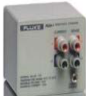
Fig. 2. Fluke 742A 1 \Omega standard resistor.
