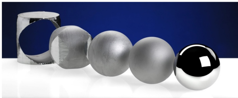
Figure 4. Steps for manufacturing nearly perfect silicon spheres.
