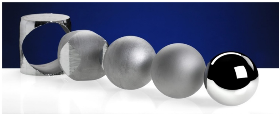
Figure 4. Steps for manufacturing nearly perfect silicon spheres.
