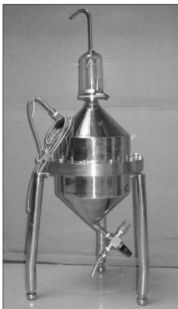
Fig. 1. Image of the 20 L transfer standard
