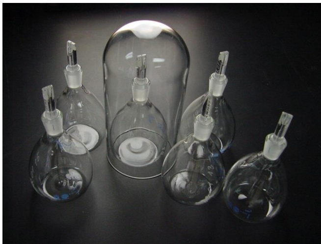
Fig. 2. Image of the 100 mL transfer standards
