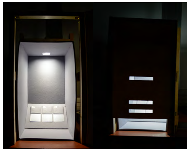
Figure 2 Observation box with samples on the exhibition plane left, with the observation shield right.
