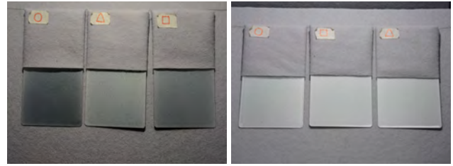
Figure 1 Samples of set Ia on the left at 0° observation, on the right at 20° observation
