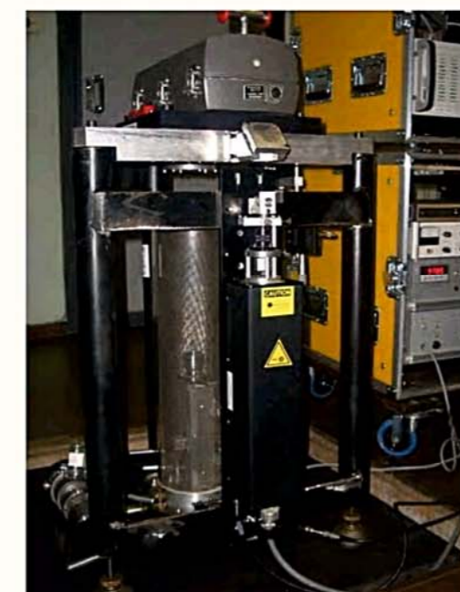
Picture of the new absolute gravimeter IMGC-02
