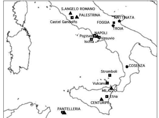
Fig. 6. Location of absolute stations in Southern Italy. Squares represent the reference stations for the relative gravity network, triangles represent the absolute stations located on the dynamic areas. Circles are the stations constituting the fundamental ties of the «Calibration line» for relative gravimeters and a station (Cosenza) settled in a seismic area.
