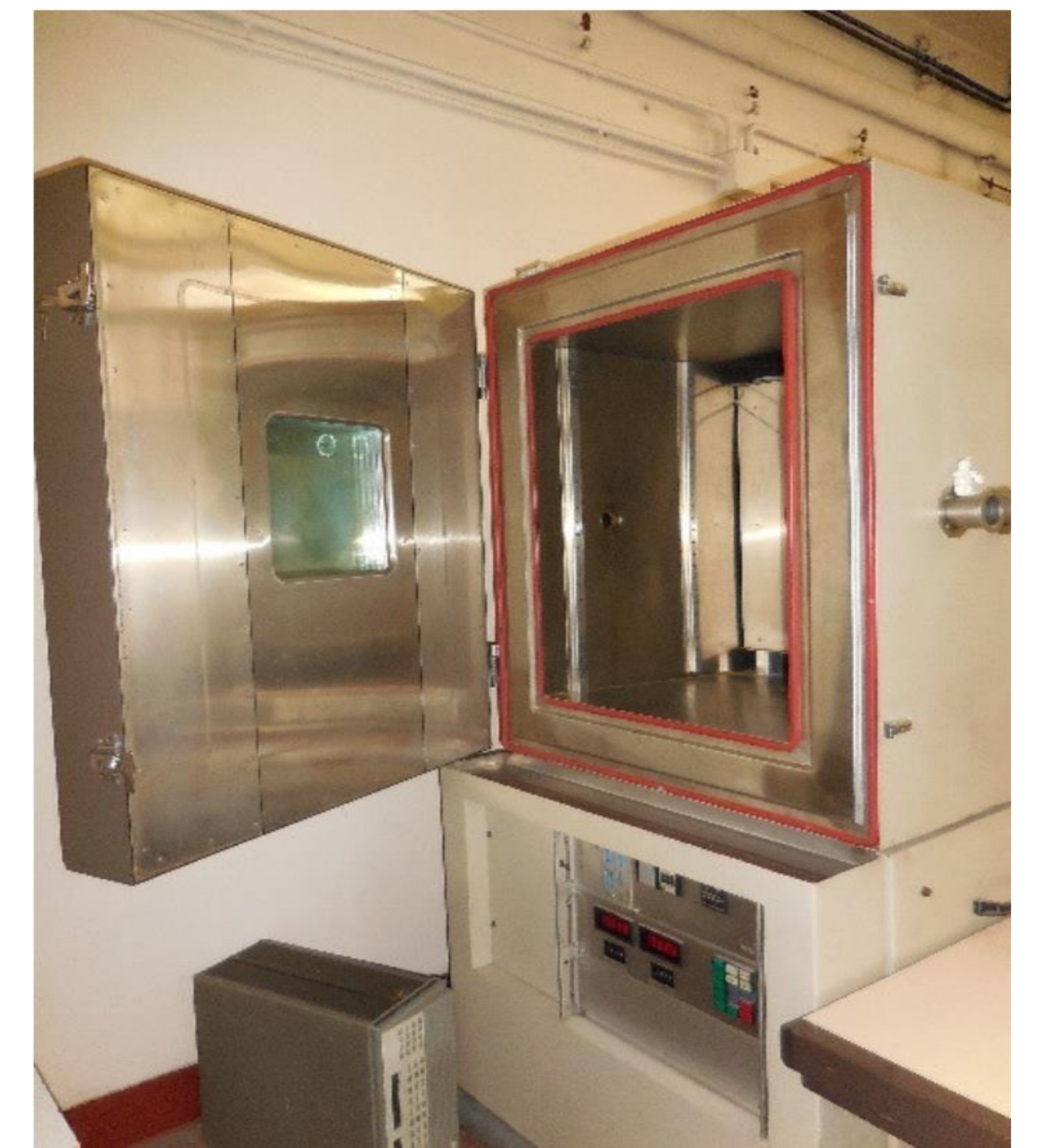
Climatic chamber Weiss Technik in operation at INRiM and used, coupled with the Kambic chamber, to test RS92 and RS41 before and after fast temperature changes.
