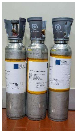
Figure 3: Examples of INRiM reference gas mixtures for CO 2 amount fraction and isotopic composition.
