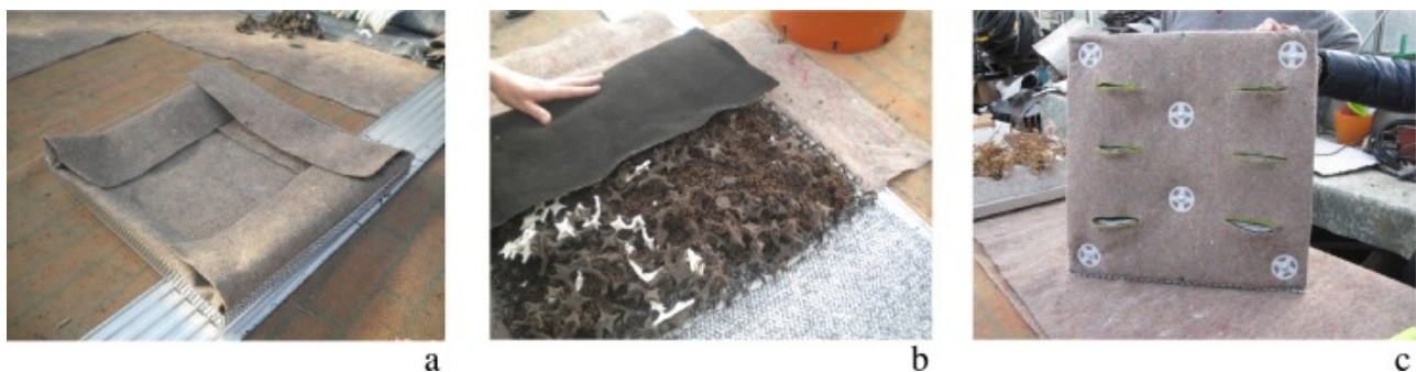
Fig. 2. Manufacturing of the final prototype. (a) Outer layer of the VGMS (recycled polypropylene). (b) Placement of the inner layer (growing medium) of the VGMS. (c) Modular box of the VGMS with pockets where the plants were to be inserted.
