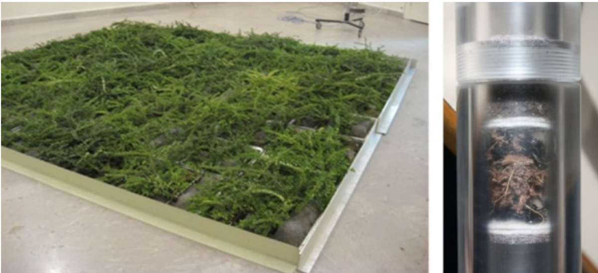
Fig. 13. Measurements of the sound absorption coefficient in the diffuse sound field (reverberation room) and in the standing wave sound field (Kundt tube).
