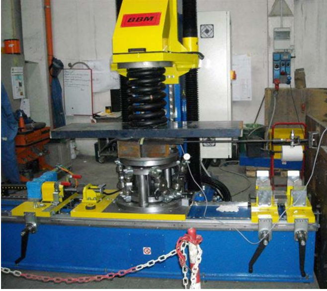
Figure 5. The second multicomponent spring testing machine by BBM during machine verification tests.
