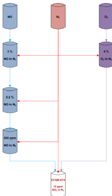
Figure 2. Preparation scheme for the mixtures
