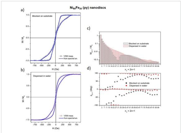
**Figure 4.** Panels (a) and (b): hysteresis loops measured on permalloy nanodiscs in quasi static conditions; (a) nanodiscs still attached to the substrate; (b) nanodiscs dispersed in water; panels (c) and (d): comparison between the amplitudes and phases of the spectral harmonics for blocked and dispersed nanodiscs.
