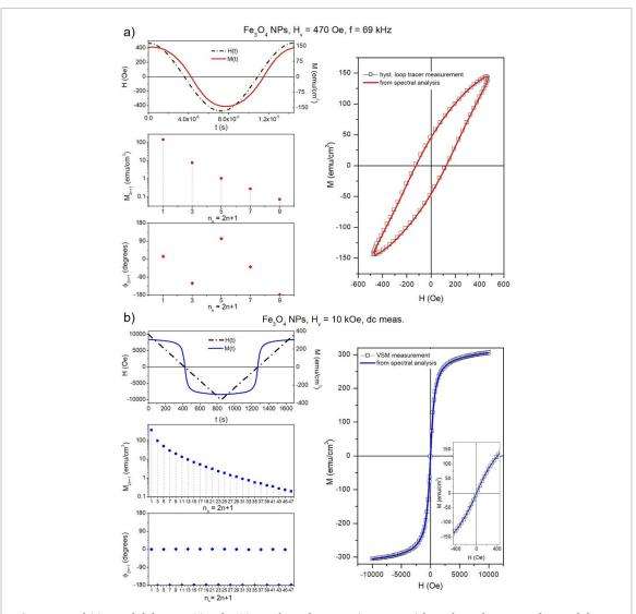
**Figure 1.** Panel (a)—top left frame: H(t) and M(t) waveforms for magnetite nanoparticles at f = 69 kHz; centre/bottom left frames: amplitudes and phases of the significant spectral harmonics of magnetization; right frame: hysteresis loop at the same frequency (open symbols: measurement; full line: reconstruction from spectral harmonics. Panel (b): the same as in (a) for the same magnetite nanoparticles measured in quasi-static conditions.
