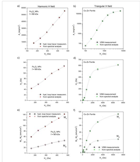
**Figure 3.** Agreement between measured and reconstructed hysteresis loop's parameters for magnetite nanoparticles at f = 69 kHz and for Co-Zn ferrite particles measured in quasi static conditions: (a) and (b) hysteresis loop's area, (c) and (d) coercive field; (e) and (f) vertex magnetization and magnetic remanence.
