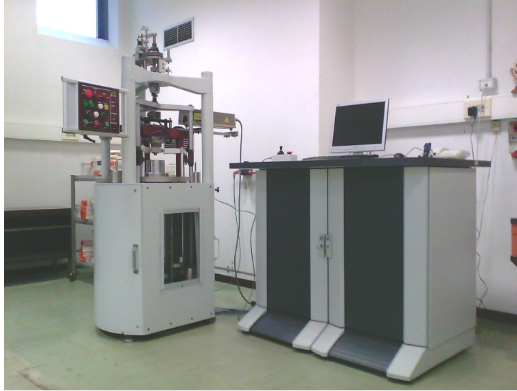
Figure 2: Primary Hardness Standard Machine at INRiM
