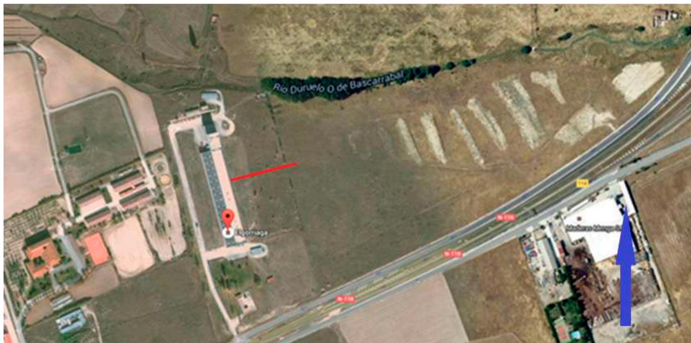
Figure 2. Real aerial view (©Google, 2016) of the selected site. The sensors are positioned along the red line, with a total length of 100 m, as described in the lower panel of Figure 1. The reference thermometer is placed at 100 m from the building. The blue arrow indicates the direct of north.
