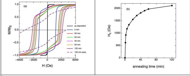
**Figure 2: (a)** Selected in-plane hysteresis loops (except for the magenta dashed line, which corresponds to the out-of-plane hysteresis loop of the 120 min annealed sample) and **(b)** coercive field as a function annealing time for  $Fe_{56}Pd_{44}$  thin films. The line is a guide to the eye.
