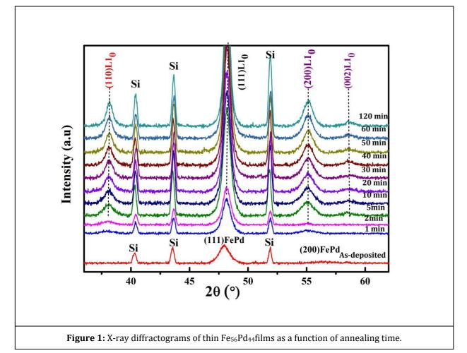
**Table 1** summarizes the lattice constants of the fcc (disordered) and  $L1_0$  (ordered) phases deduced from the X-ray diffractograms using the Bragg equation. The lattice parameter of the disordered FePd phase has been calculated from the (111) peak, whereas for the ordered  $L1_0$
