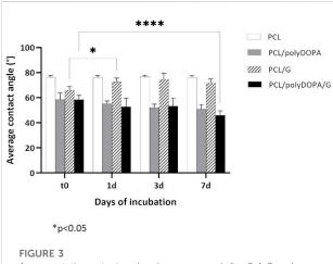
Average static contact angle values measured after 0, 1, 3, and 7 days (t0, 1d, 3d, and 7d) incubation in PBS at 37°C for PCL, PCL/polyDOPA, PCL/G and PCL/polyDOPA/G model films. Reported data are the average values  $\pm$  standard deviation (n=9). \* p-value <0.05.
