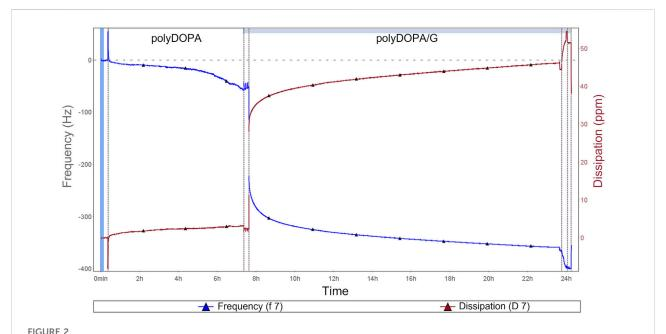
QCM-D analysis during polyDOPA/G deposition: blue curve refers to frequency, while red curve represents dissipation as a function of incubation time. All the phases of functionalization are displayed, including initial sensor preconditioning as well as washing steps after polyDOPA coating before G deposition.
